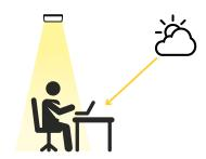
With insufficient natural light, the sensor will switch on the light when a presence is detected.
