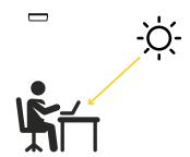
With sufficient natural light, the light will not switch on even if a presence is detected. Manually adjustable light level.
