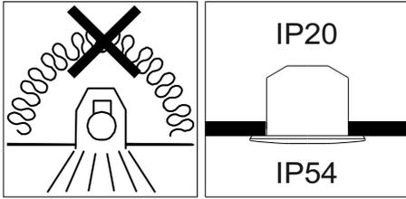
Luminaires not suitable for covering with thermally insulating material
