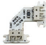
42AA05EL 2 ways 90° electrified connector.
