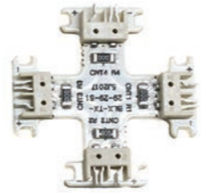
42AA07EL 4 ways electrified connector.
